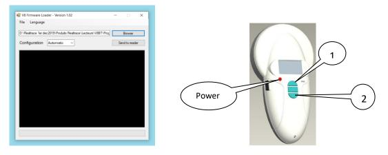
Start the V8 by holding down the Up (1) and Down(2) keys for a few seconds while pressing Power. Release the keys.
